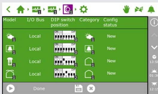
Figure 4-2: Smart Switches found in the system.
