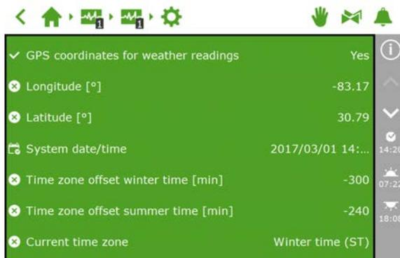
Figure 4-5: The 'GPS coordinates for weather readings' setting is enabled
